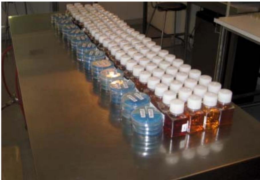
Above, beer samples and media bar-coded using the Yeastman computer system await testing last year. The barcoding eliminated any possibility of bias, as the name of the brewery was not included on the sample. At right, the Perkin Elmer GC-Headspace auto-sampler is filled with over 100 vials for analysis during Big QC Day at White Labs.
